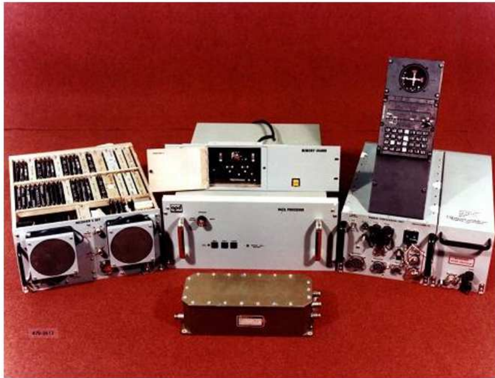
1977 - The Magnavox X-Set was the first to track a GPS signal from space (NTS-2 Satellite GPS Experimental Satellite)
